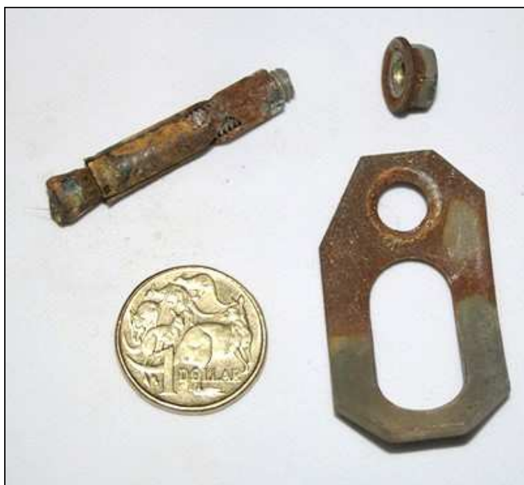
This picture shows the state of the bolts removed from ' The Dynabolt of Death '
